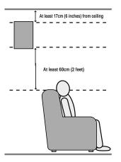
speakers should be located so that the bottom of the cabinet is at least 60cm (2 feet) higher than the listeners' ears when the listeners are seated in the desired area.
